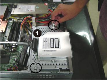
Unscrew the HDD cover plate.
