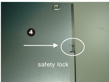
To replace the cover, slide the cover forward and make sure the safety lock fits firmly.
