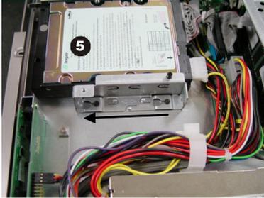
Push the HDD bracket forward to secure the HDD.
