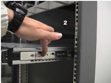
The system will be locked halfway while pulling it out. Pull forward the locking tabs on both sides of the chassis rails to unlock the tab. You may now remove the system from the rack.
