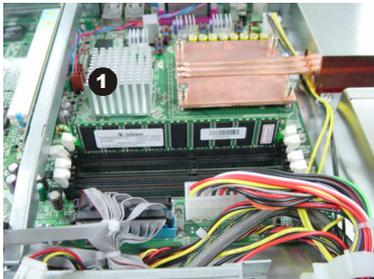
Locate the DIMM slots on the mainboard.
