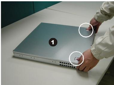
Locate the release buttons on the chassis cover.
