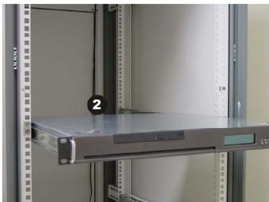
Align the chassis rails with the rack rails, and then push the system into the rack fully
