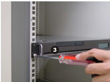
Secure the system with the screws.
