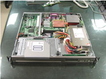
The installation of the heatsink and fan duct is now completed.
